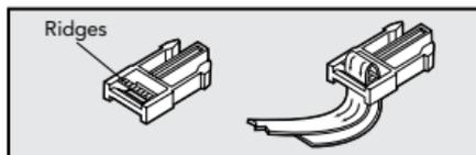
The ridges must be facing up; the collar will slip if it is not properly threaded.
